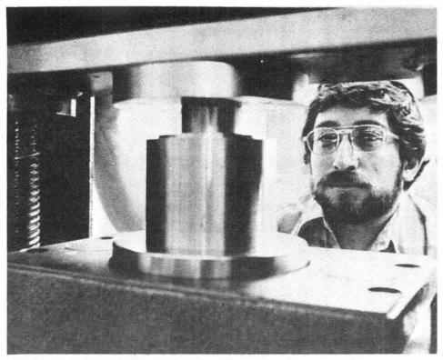
PROCESS TECHNOLOGY ANALYSIS—Above, Tino Casaus makes measurements of mechanical properties of materials using Instron instrument. At right, Jake Young operates scanning electron microscope. Image shows angled surface of solar collector material magnified 300 times.
